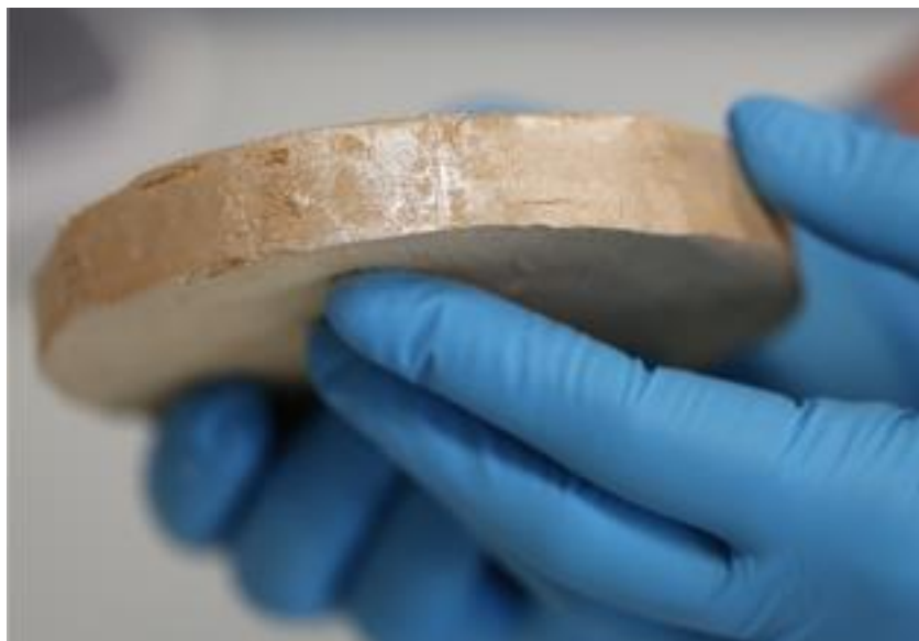
Figure 1. Picture of the bulk ceramic green body with nacre-like microstructure obtained by the fabrication route developed in the SCCER project.
