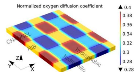
3D simulation of a gas diffusion layer with patterned wettability for improved oxygen diffusivity [3].
