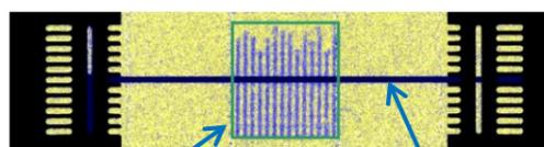
Neutron imaging of the water distribution in a laboratory test cell (4 cm<sup>2</sup>) using the proposed concept [2].
