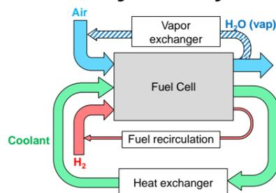
A vapor exchanger for humidification and a separate coolant loop are required.
