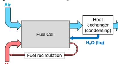
Humidification and cooling by water injection, simplifying the system and removing costly components. The distribution of injected water is challenging.
