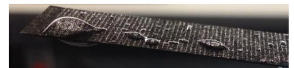
Within the SCCER Mobility, we use a novel material with patterned wettability developed at PSI [1]. It allows to finely distribute the water without blocking the access of hydrogen and air.
