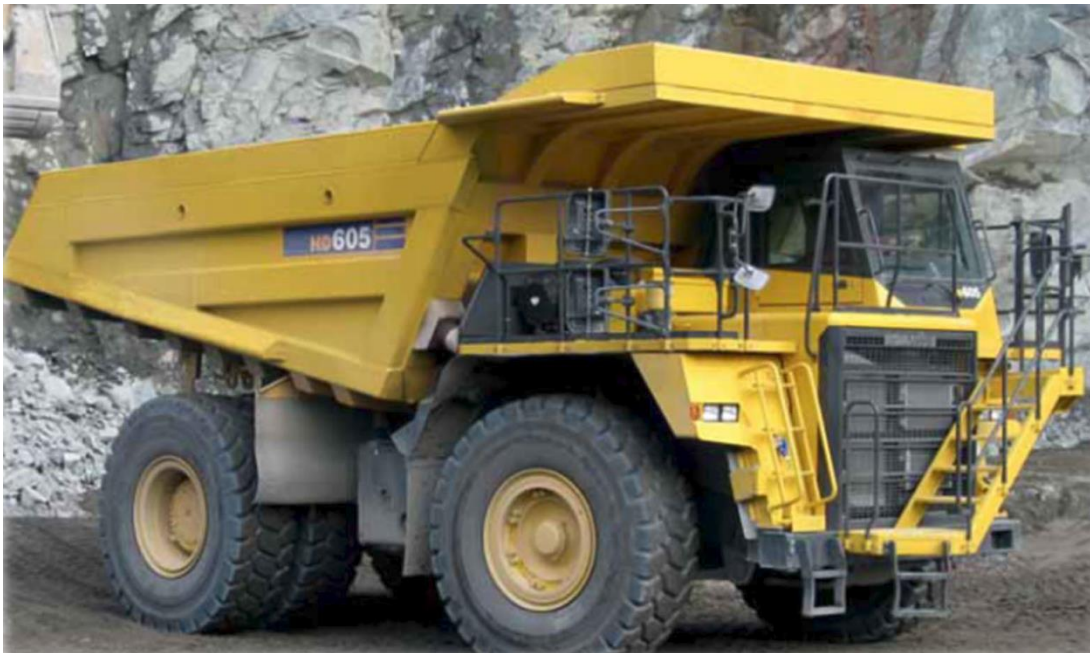
Komatsu HD605-7 Elektro: 111 tons fully loaded, 60 tons limestone
