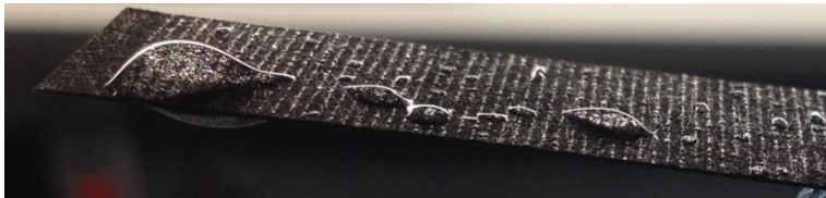
Figure 1: Optical photograph showing the surface of modified, patterned gas diffusion layer (porous carbon fibre sheet) for use for evaporative cooling in fuel cells.
