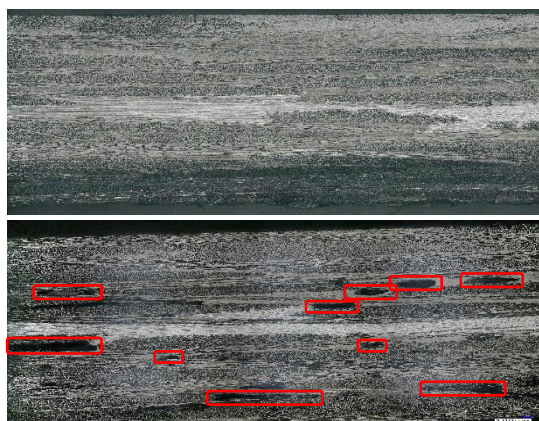
Figure 1. Micrographs of two plates after impregnation with different process parameters (porosities are circled in red).
