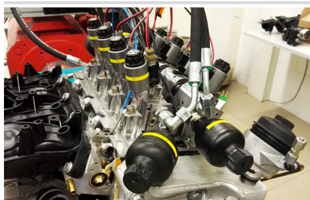
Fig. 1: Fully variable valve train on engine test bench.
