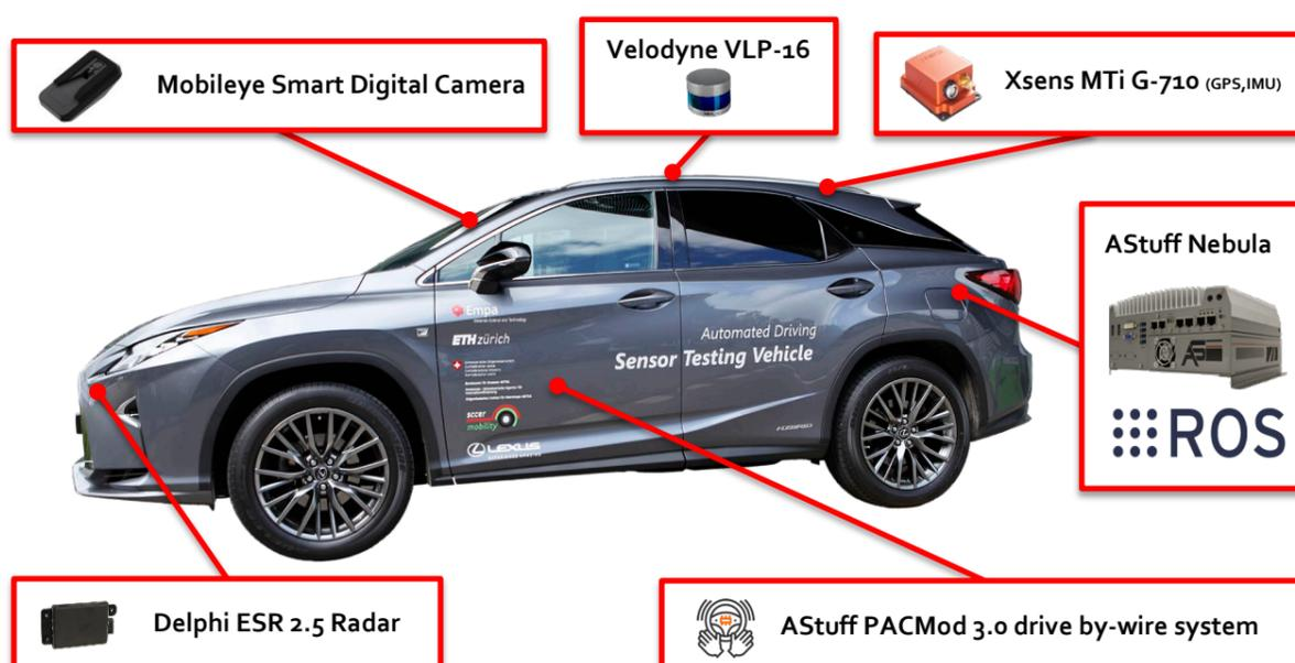
Figure 6: Lexus RX 450h with autonomous driving sensor and computing equipment [3].
