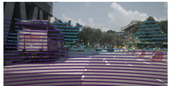
Figure 4: LIDAR point cloud and front camera image fusion (data from [2]).
