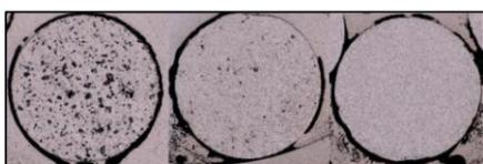
Fig. 6: Ø 10 mm PET samples with increasing throughput
