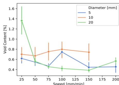
Fig. 7: void content of pultruded samples
