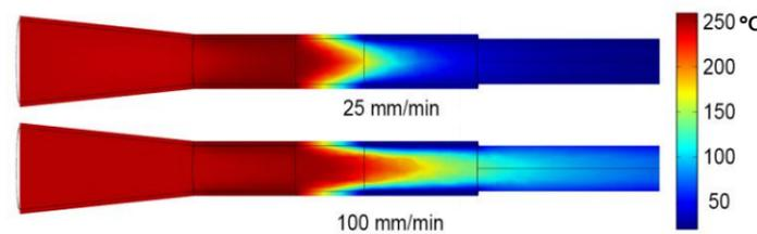
Fig. 3: temperature distribution inside pultrusion die
