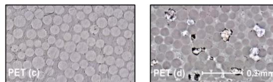
Fig. 8: PET samples before (c) and after voltage tests (d)
