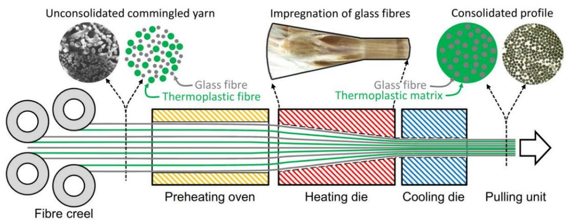
Fig. 2: Thermoplastic pultrusion process using commingled yarns
