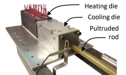
Fig. 4: pultrusion set-up
