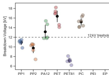
Fig. 9: Breakdown voltages for different polymers
