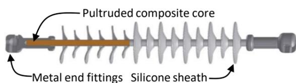
Fig. 1: composition of composite insulator
